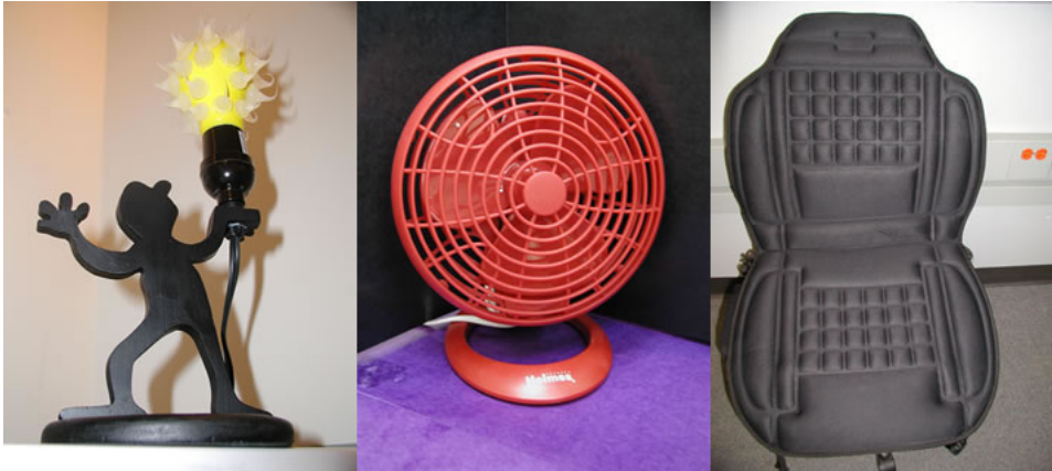
Figure 1: Everyday objects that have been imbued with computational power to enable them to convey information using the Real World Interface Toolkit. From the left to right, they are the infoLAMP, the dataFAN and the hapticCHAIR.
